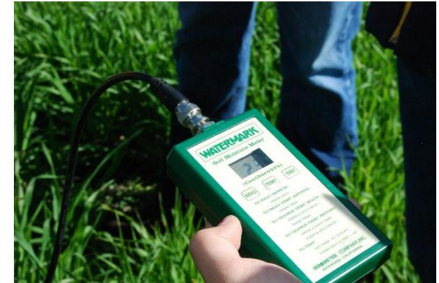
Figure 82 Soil moisture meter. © Wikimedia https://commons.wikimedia.org/wiki/File:Irrigation90_(38829459642).jpg
