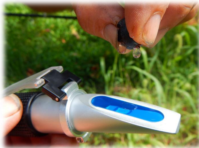
Figure 12 Using of refractometer to measure the sugar content © https://mountainviewvineyard.com/
